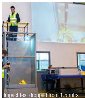
Impact test dropped from 1.5 mtrs
