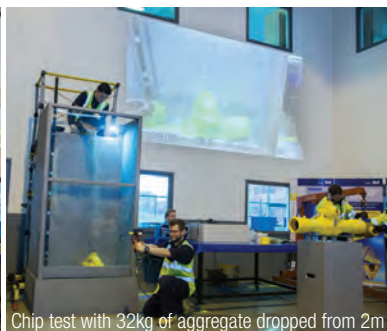
Chip test with 32kg of aggregate dropped from 2m
