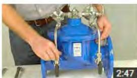
**Maintenance of the main valve of an AVK control valve**
