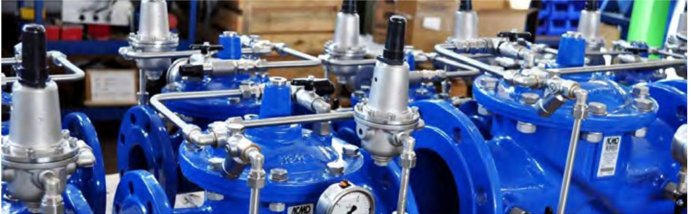
A restriction orifice, inside of the “strainer” located upstream of the control chamber, will limit the flow rate. A restriction orifice located just downstream of the filter will limit the flow rate. The valve will open if the flow rate allowed through the control pilot, located downstream of the control chamber, is greater than the flow rate allowed through the restriction orifice.
