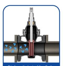
This forms the basis of the effective double block, and the gas bleed plug enables the void in the valve's center to be vented to atmosphere creating the double block and bleed which facilitates safe working on the network downstream of the valve.
