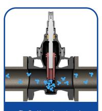
The Donkin wedge gate seals on the sides of the valve well at the foot. Even so, as the valve is closed the increased velocity of gas through the closing gap flushes any debris from the well.
