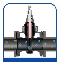
When open, the Donkin 555 gate rests completely outside the flow of gas for optimal flow and the metallic gate means reduced wear over time from any particulates in the gas flow.
