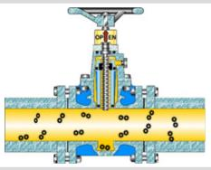
The Donkin wedge gate seals on the sides of the valve well at the foot. Even so, as the valve is closed the increased velocity of gas through the closing gap flushes any debris from the well.
