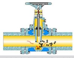
This forms the basis of the Donkin valve's effective double block and with the gas bleed plug enable the void in the valve's centre between the faces to be vented to atmosphere creating the Double Block and Bleed which facilitates safe working on the network downstream of the valve.
