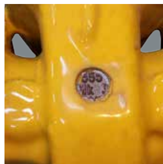
ADHESION - PULL OFF TEST
