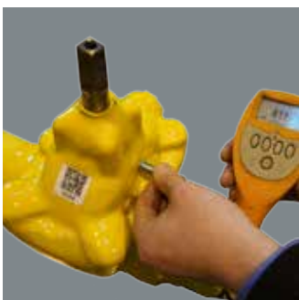
MINIMUM COATING THICKNESS
