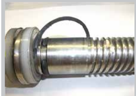
Damaged spindle thread and O-ring
