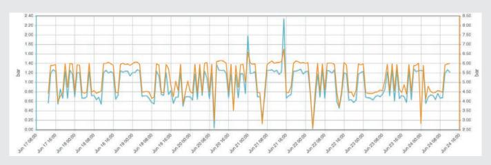
This graph show the pressures of two different ARISENSE air valves simultaneous over an eight-day period, hourly. These can then be inspected to see if there is any irregularities between certain air valves suggesting a possible burst/leak.
