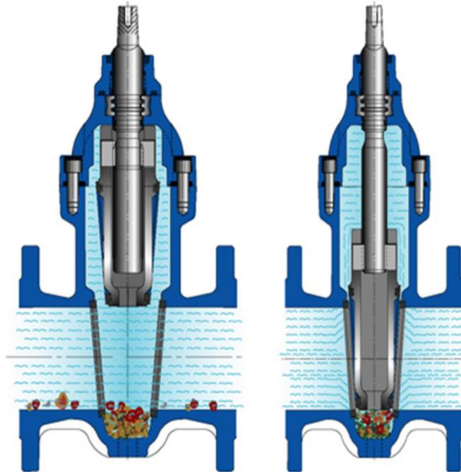
*Figure 2 – metal seated gate valve (sump at base of valve bore)*
