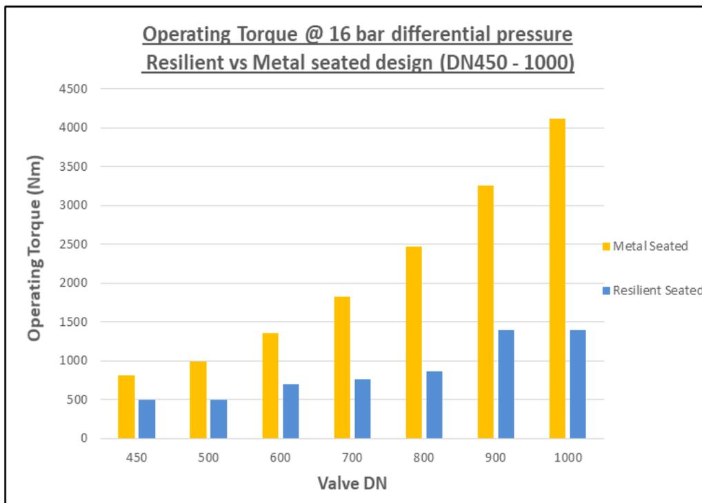
*Graph 1 – comparison of operating torques for metal vs resilient seated gate valves*
