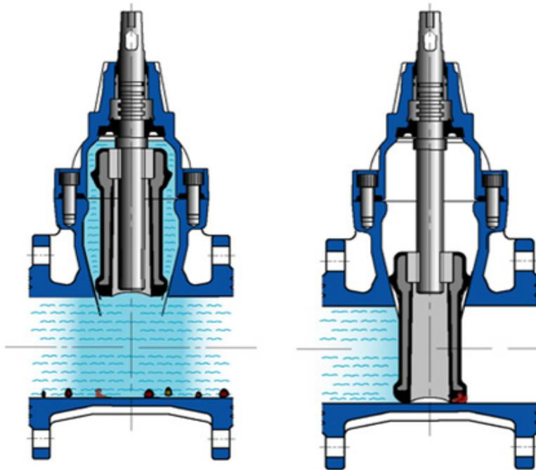
Figure 1 - resilient seated gate valve (smooth base on valve bore)
