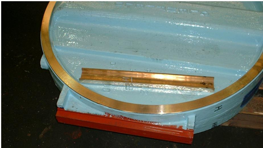
*Figure 3b – extruded aluminium bronze shoe fixed onto metal seated gate valve wedge*
