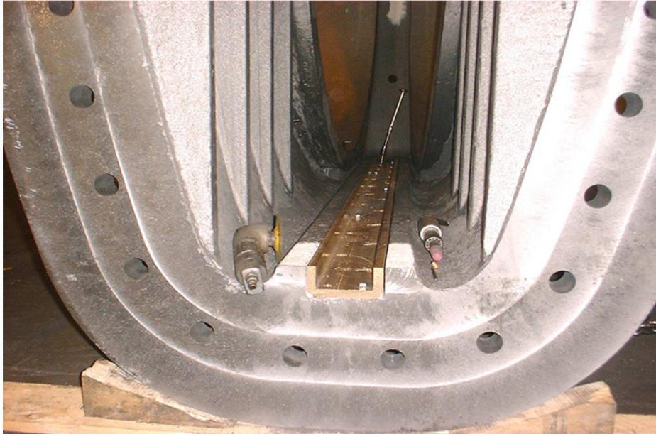
*Figure 3a – extruded aluminium bronze channel fixed onto metal seated gate valve body*
