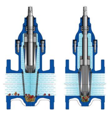
Figure 2 – metal seated gate valve (sump at base of valve bore)
