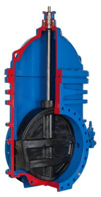
Figure 4 – cross sectional view of large resilient seated gate valve with vulcanised wedge
