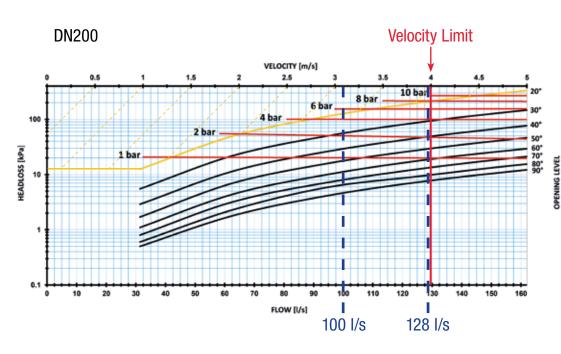
**NOTE:** The maximum recommended velocity is 4 m/s as per EN1074.
