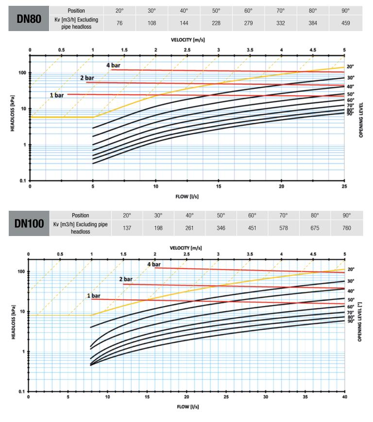
For flow control, valves should only be used if the plug is open to 20° and over, they should not be used for control at an angle lower than this as represented on the graphs by the orange lines.
