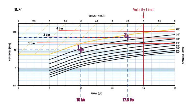
**Point 1** – At a flow of 10 I/s and pressure loss of 10 KPa the valve should be just over  $30^{\circ}$  open.
