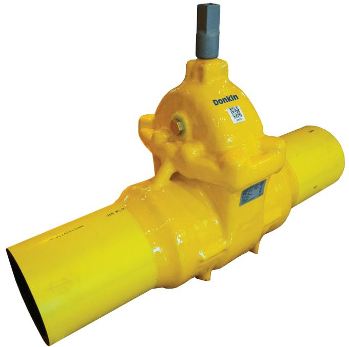
**REDUCE VALVE WRAPPING** - The Polyurethane coated, PE tailed, Series 555 can be installed **without** any further corrosion protection required, so it's just a case of install, record and backfill. Valves with flanged ends have fully protected valve bodies but will still need to be wrapped on the connecting flanges to ensure that the connecting bolts are fully protected. This is a **major saving** on both models when compared to wrapping the whole valve.
