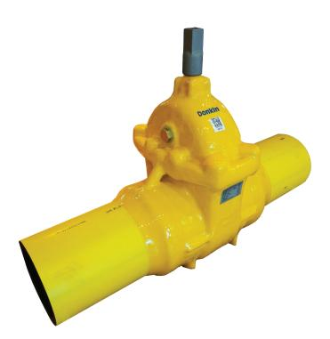
**REDUCE VALVE WRAPPING** - The Polyurethane coated, PE tailed, Series 555 can be installed **without** any further corrosion protection required, so it's just a case of install, record and backfill. Valves with flanged ends have fully protected valve bodies but will still need to be wrapped on the connecting flanges to ensure that the connecting bolts are fully protected. This is a **major saving** on both models when compared to wrapping the whole valve.
